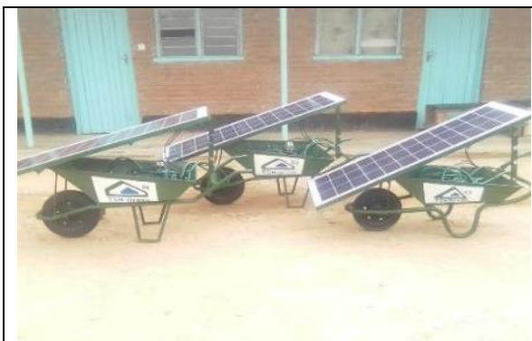
A pump, panel, hose and cable mounted on a wheelbarrow. It is easily transported to distance fields for irrigation
