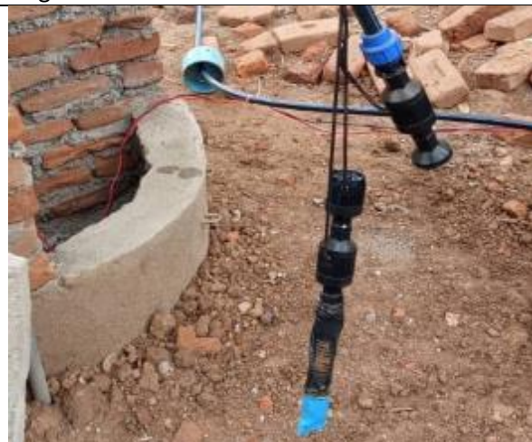
Sometimes the top cap of the pump model 38 can become loose, especially if more pumps are mounted in series
