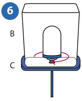
Screw the Tulip filter element with the rubber ring and the fast flow hose into the upper bucket (B) and lower lid (C). Make sure the rubber ring is between the filter element and the bottom of the bucket.
