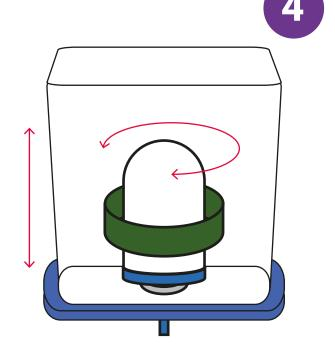
After some time, the flow rate reduces. Take the scrub pad (M) and carefully scrub the filter element to remove a very small layer of the ceramic material.
