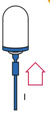
Attach the fast flow hose (I) to the nipple of the Tulip filter element (F) and make sure it is tightly fastened.
