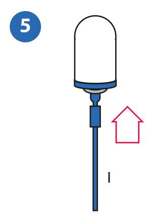
Attach the fast flow hose (I) to the nipple of the Tulip filter element (F) and make sure it is tightly fastened.
