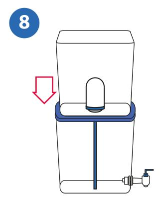
Place the upper bucket, with the lid of the lower bucket, Tulip filter element and fast flow hose onto the lower bucket.
