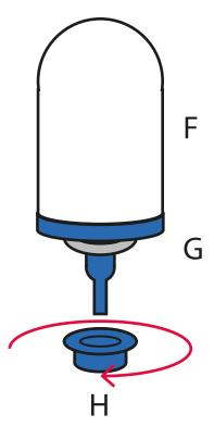
Remove the filter nut (H) from the Tulip filter element (F). Leave the rubber ring (G) on the filter element.
