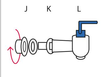
Unscrew the tap nut. Leave one rubber ring (K) on the tap (L) and remove one (K).
