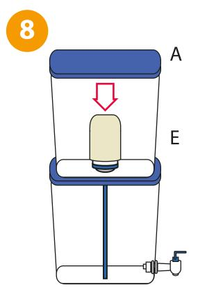
Put the pre-filter (E) over the filter element and place the upper lid (A).
