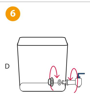
Screw the tap with one rubber ring through the hole on the inside of the lower bucket (D) and one outside. Fasten the tap tightly by using the tap nut (J).
