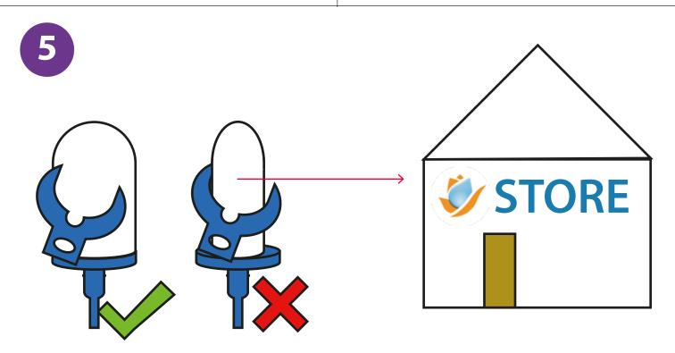
With the plastic end of life indicator (N) you can measure when your filter element has to be replaced. When the end of life indicator (N) fits around the thinnest part of the filter, the filter can no longer make the water safe to drink and must be replaced.
