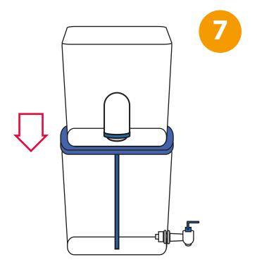
Place the upper bucket, with the lid of the lower bucket, Tulip filter element and fast flow hose onto the lower bucket.
