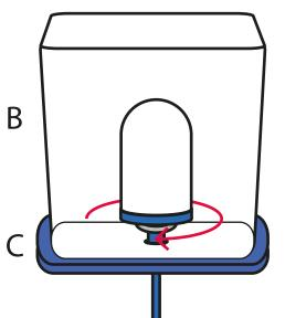
Don't push the filter element, but turn it to avoid breakages and ensure tight fastening.
