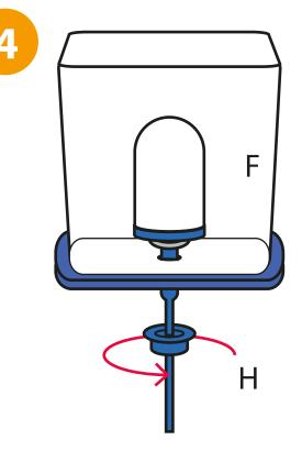
Fasten the Tulip filter element (F) by using the filter nut (H).
