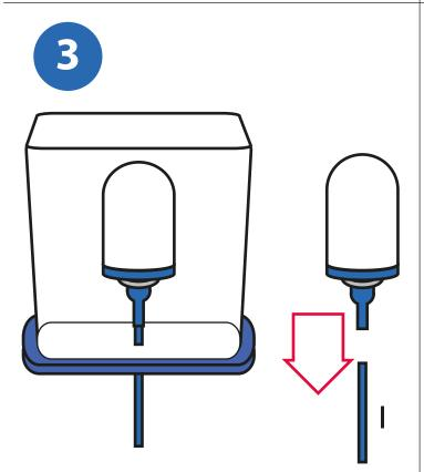
Take out the ceramic candle element. Pull the fast flow hose (I) off the filter element.
