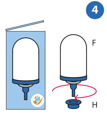
Take a new filter element out of the box. Remove the filter nut (H) from the Tulip filter element (F). Leave the rubber ring on the filter element.
