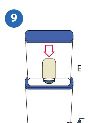
Put the pre-filter (E) over the filter element and place the upper lid (A).
