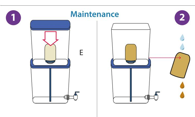
To protect the filter element against clogging, the filter element is covered with a washable pre-filter (E).
