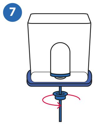
Fasten the Tulip filter element (F) by using the filter nut (H).
