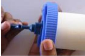
2. Cut the hose near the nozzle with a knife.
