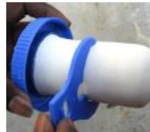
With the plastic sensor you can measure when your filter has to be replaced. When the plastic sensor fits around the thinnest part of the filter, the filter is no longer safe to filter the water and it has to be replaced. Ask your local supplier for the replacement filter.
