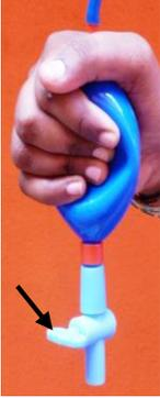
2. Put the filter back in the water, wait until the bulb is filled again with water and open the tap.
